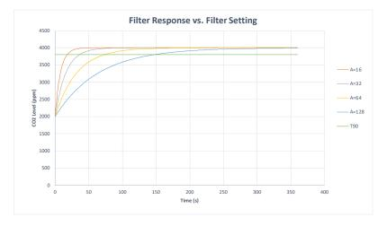
The graph above shows the effect of the filter on response times. Increasing the filter setting increases the measurement output response time.  $T_{90}$  is the time to 90% of reading. The ExplorIR®-W takes 2 readings per second.
